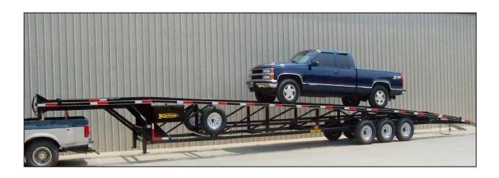
Correct; even with a single vehicle make sure the load is evenly distributed! Move slowly through turns and unlevel ground to avoid rollover!!
