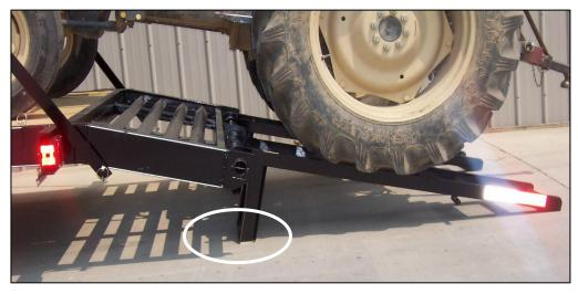
During the loading process, the dogleg should touch the ground in order to support the weight of the equipment being loaded.
