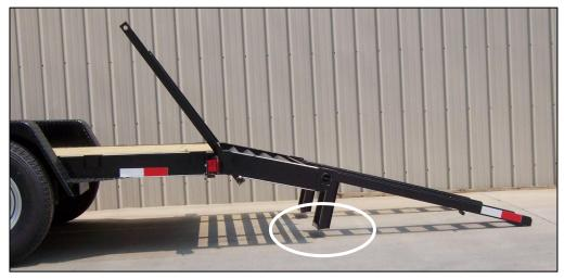
An empty trailer that is level with the ground will have the proper distance between the ground and ramp dogleg.
